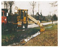
projects without interrupting traffic flow. It also features the Gradall 5-way boom, lifting, digging, tilting, swinging and telescoping with simultaneous movement of the boom improving cycle time. For outstanding versatility, most of the attachments used with the previous Gradall G440 and G3W can be utilized . . . ditching buckets, grading blade, pavement-removal bucket, trenching buckets, and single-tooth ripper.
